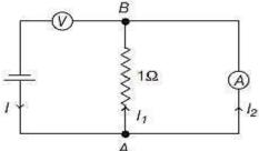
Let I = current through cell, then potential drop read by voltmeter is  $V = I \cdot R_V$  (this is reading of voltmeter) Where,  $R_V$  is the resistance of voltmeter In loop AB,
