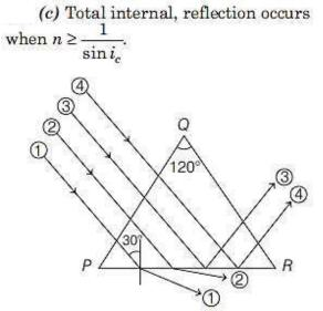
In given situation, angle of incidence of each of ray is  $30^\circ$  over face *PR*.
